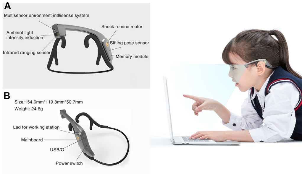
Figure 1. Function module diagram and photo demonstration of the Eye-Use Monitor.
